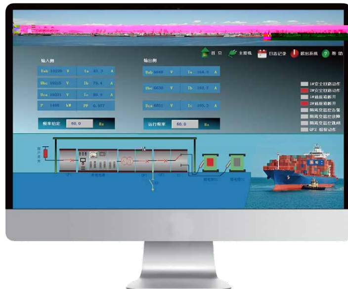
Shore Power Monitoring System
